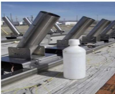
Simulator Projectile Airburst Liquid (SPAL) system
